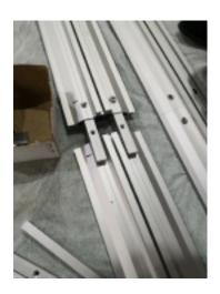
2. 90degree corner joint to install the frame by square or rectangle.
